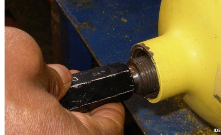
Checking the cylinder neck thread with a threaded gauge
