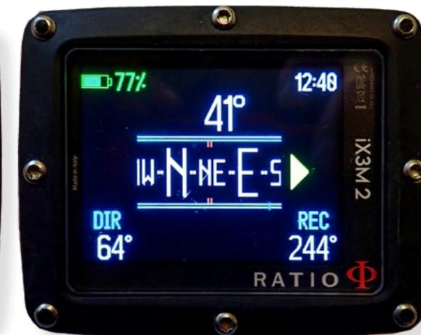
The compass on the Ratio iX3M 2 dive computer shows direction on and off course.
