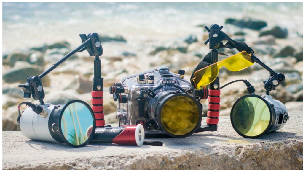
My Ikelite fluoro set-up. Filters are easily taken on and off underwater to allow for normal photography too.
