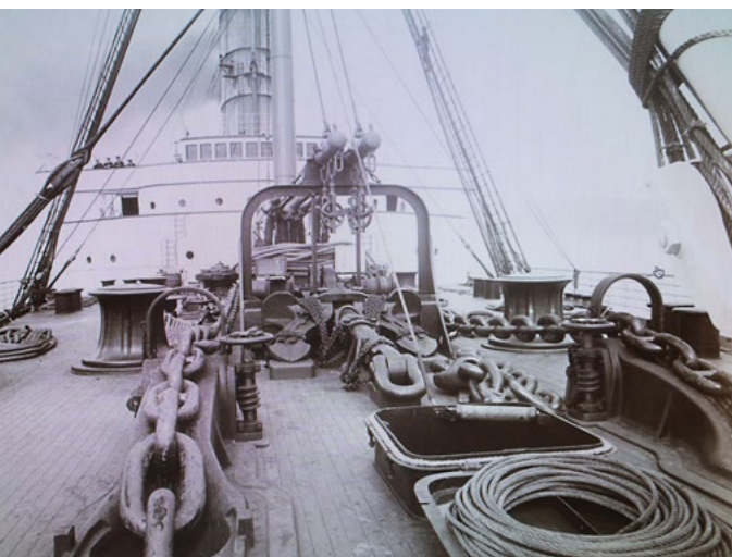
Historical photo showing the anchor chain and winch on the Lusitania
