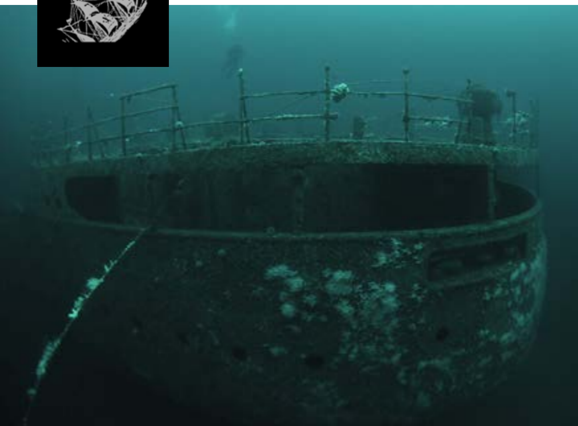
AFT AND FORE: The stern (below) is very much intact, while the bridge (right) and wheelhouse have partly collapsed over the years
