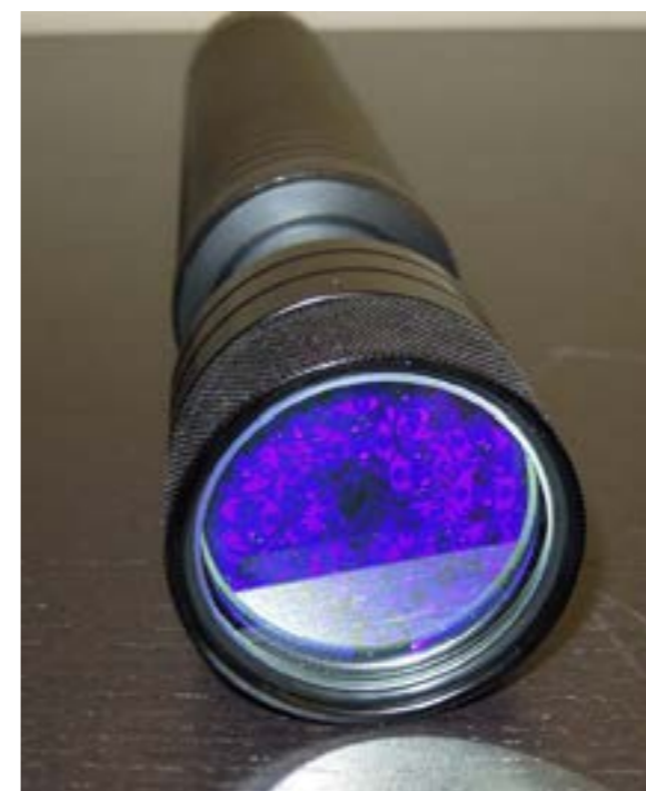
The author's torch with 18 blue Cree LEDs and a dichroic blue filter
