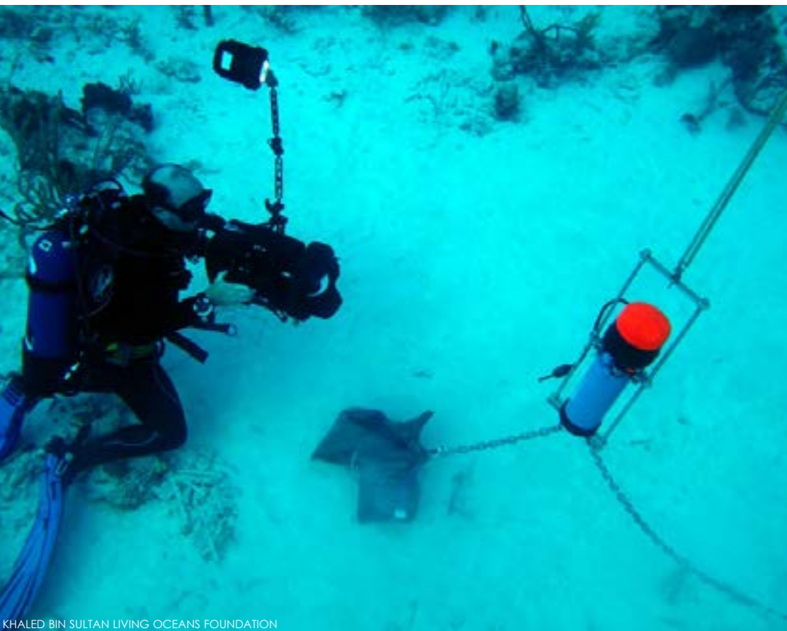
Allan filming current meter deployment
